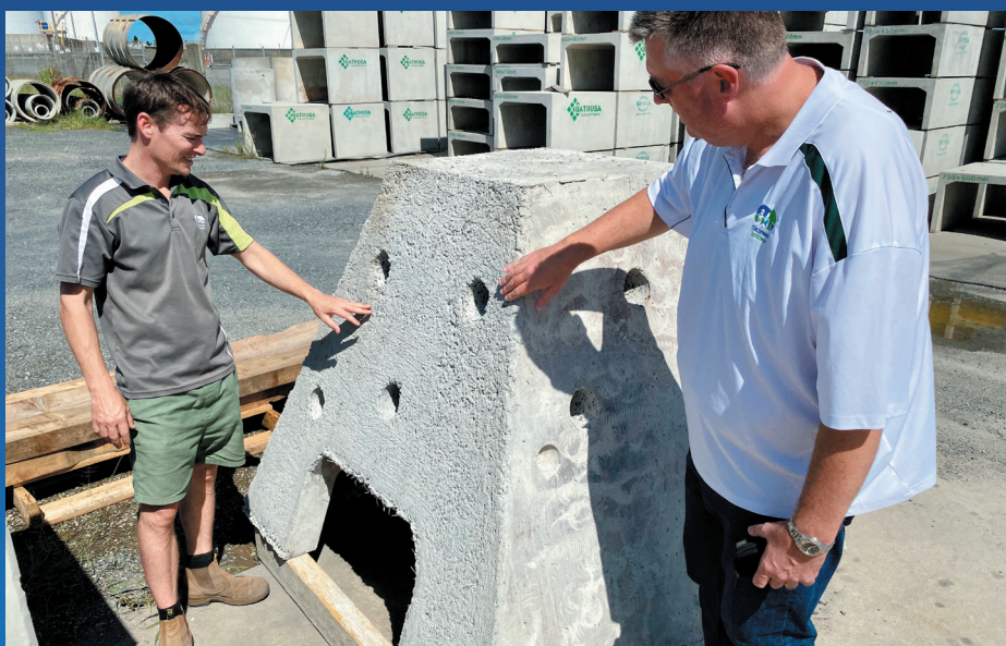
Prototype 'Pyramid' reef module showing surface roughness and juvenile fish habitat
